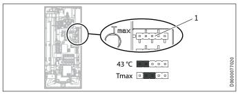
1 Jumper for anti-scalding protection setting
