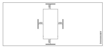
► Maintain the minimum clearances to ensure trouble-free operation of the appliance and facilitate maintenance work.
