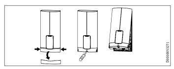
▶ Open the appliance by holding the fascia at the side and pulling forwards away from the appliance cover. Undo the screw. Pivot open the appliance cover.
