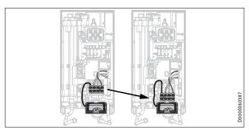
► Reposition the mains terminal further downwards. To do this, undo the fixing screw. Secure the mains terminal in place.
