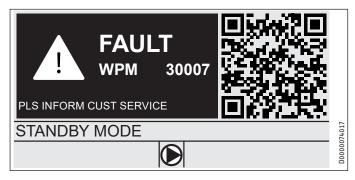
The fault is shown on the display with a fault number. Use the fault number to find more information about the fault in the message list.
