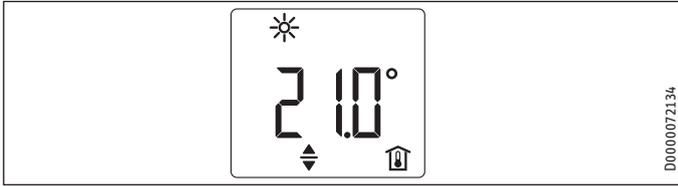
The default display is continuously displayed. If no user action is performed for longer than 20 seconds while in the menu, the appliance automatically switches to the default display.
