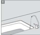
If there is no installation mistake or leakage keep the faucet open for 10 minutes to bring residual particles and air out of the unit.
