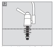
Insert the rubber washer from beneath the sink and fix the faucet in place.
