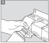
Press the push button and rotate the filter to eject.
