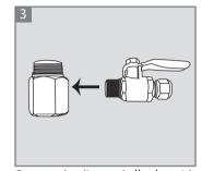
Connect the diverter ball valve with the nipple (use teflon-tape).
