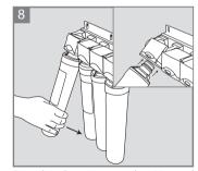
Bring the adapter in upward position and insert the filter. A loud "click" will signal that the filter is attached properly. Bring the filter back in the normal position.
