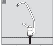
Insert the base washer to the screw beneath the faucet's main body and insert the faucet to the hole.
