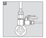
Open the diverter valve under the sink slowly. Check the whole system for water leakages.
