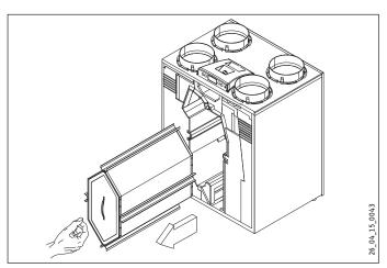
► Carefully remove the heat exchanger from the appliance. Avoid damaging the foam parts in the appliance.
