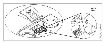
The X14 connection is used to connect an external reheater coil.
