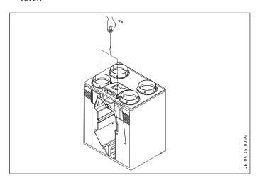
► Undo both screws securing the display cover to the appliance.
